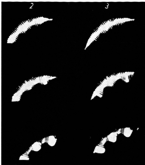
Fig. 15. Image converter pictures of shape 1 discharge (40 mtorr H_2 , B_{\max}=11 kG, with pre-ionization) for different current loop arrangements.
